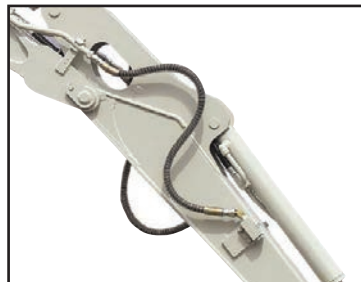
Auxiliary Hydraulic Lines
